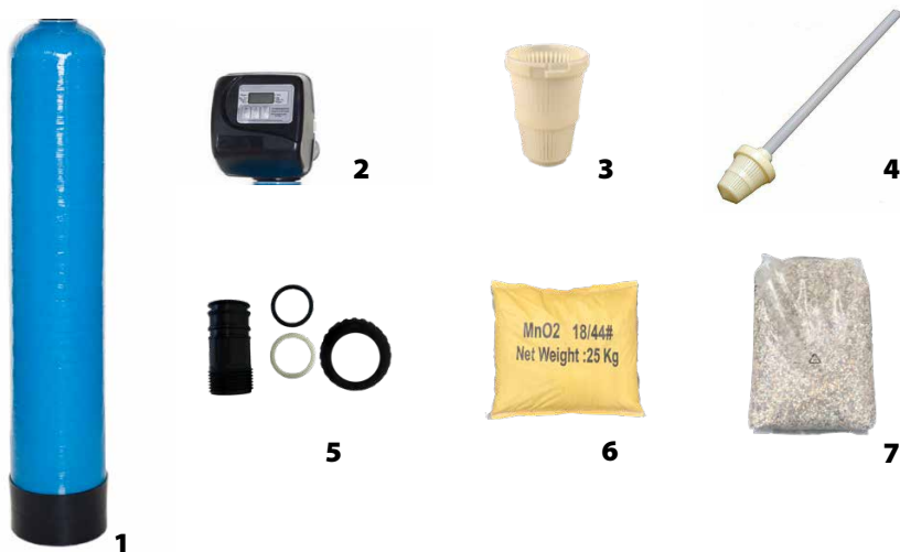
1. Vessel 2. 3-Button Clack Valve (Clack Head) 3: Distributor Basket 4: Riser Tube 5: Clack Valve-connection fittings (pack of two) 6: Activated CARBON 7: Filter Gravel
